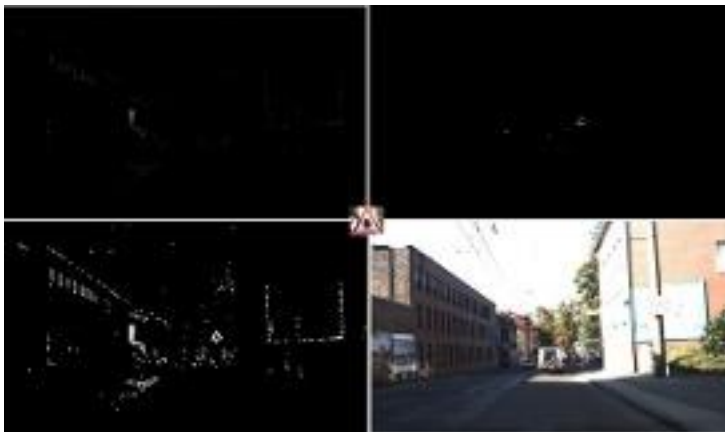
Figure 2. First line - blue mask and red mask; Second line - enhanced merged mask and original image with sign detected in a bounding box; In middle - cropped output traffic sign
