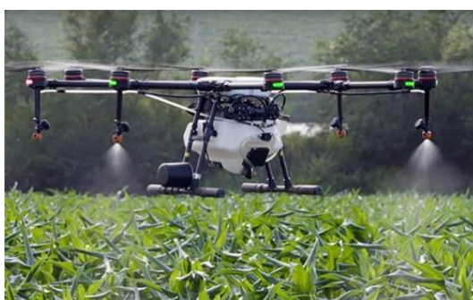
Figure 2. Drone applying spray treatment 4
